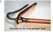
between the tube and wire were enough to allow the end to keep a grip on a sail (so the planned complication of a spring to pull on the wire proved unnecessary.
